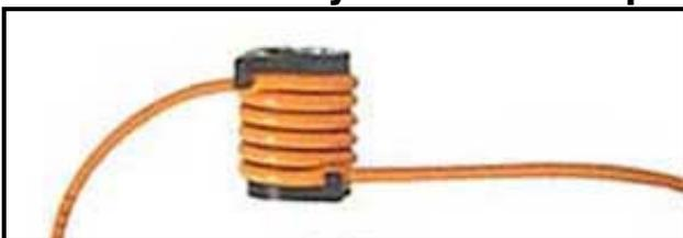
Mode filters are used to selectively remove higher order modes to attempt to simulate EMD conditions, assuming that one starts with fully filled modes. Higher order modes are easily removed by stressing the fiber in a controlled manner, since the higher order modes are more susceptible to bending losses.
